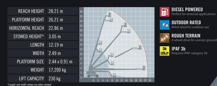
The JLG 860SJ has the ability to reach its full elevation of 28 metres in just 70 seconds - that's 40% faster than the competition. Its ease of operation and its narrow fixed width chassis makes operating in confined spaces easy.
